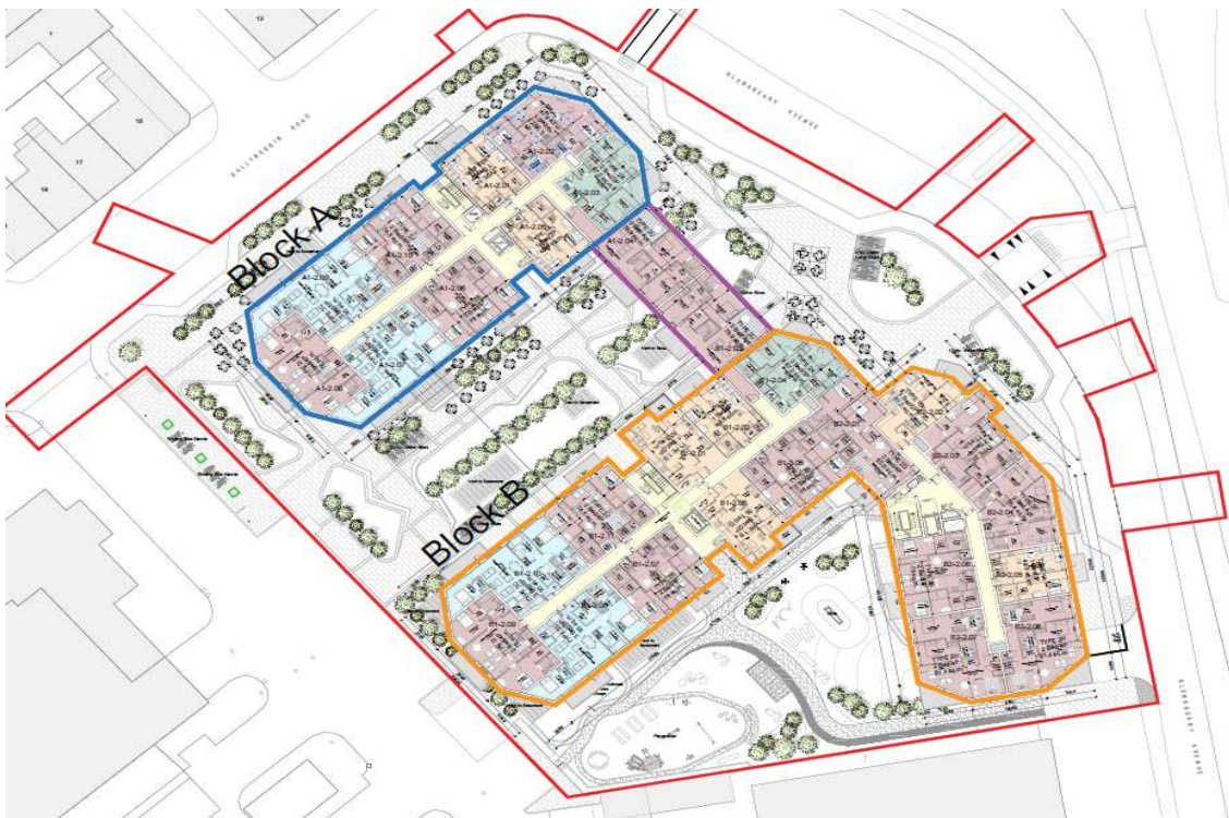
Figure 6. Phasing drawing at 1 st & 2 nd floor, Phase 1 is Block A (highlighted in blue), Phase 2 is Block B (orange), Phase 3 is the Link Bridge (purple).
