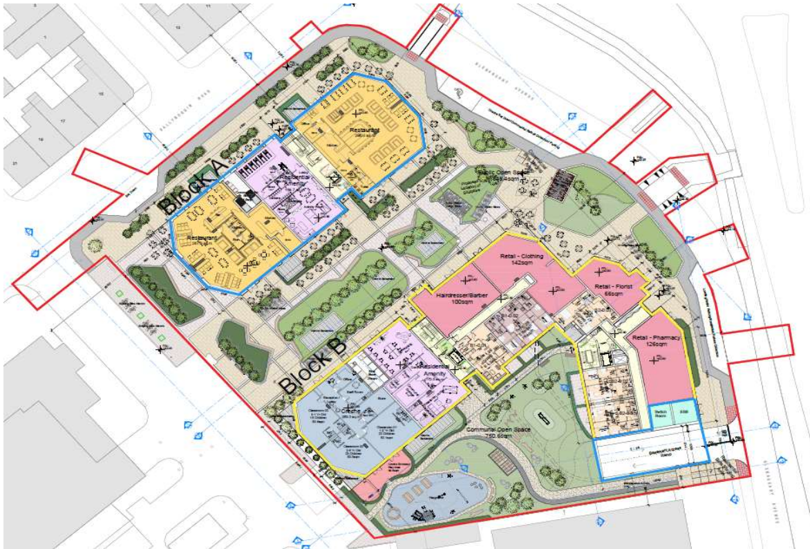
Figure 5. Phasing drawing at ground floor, Phase 1 is Block A & ESB substation (highlighted in blue), Phase 2 is Block B (highlighted in yellow).
